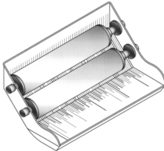
Figure 5. Rollers used in grinding/milling
