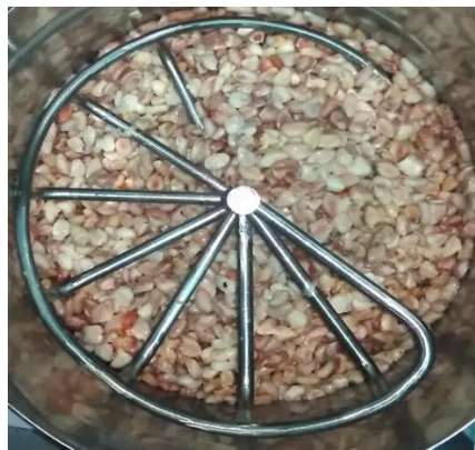
Figure 4. Cacao beans loaded in the mobile cacao bean fermenter.
