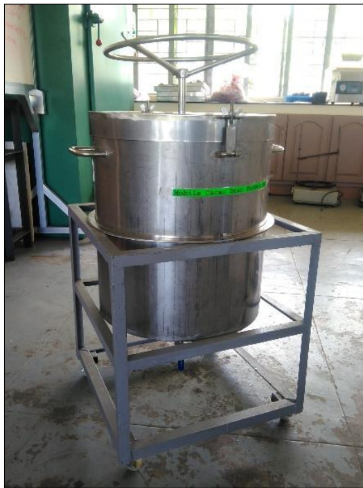
Figure 2. The fabricated mobile cacao bean fermenter
