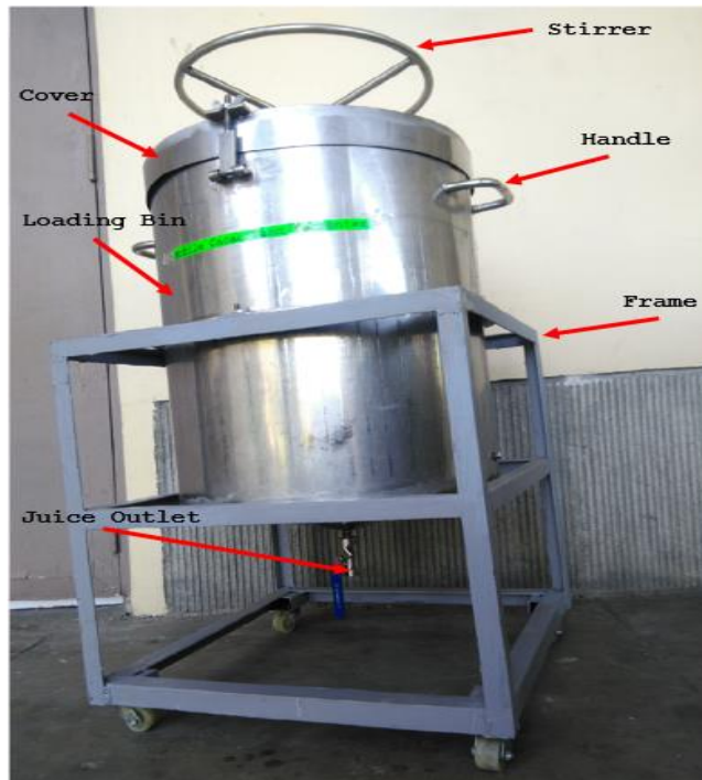
Figure 3. The fabricated mobile cacao bean fermenter
