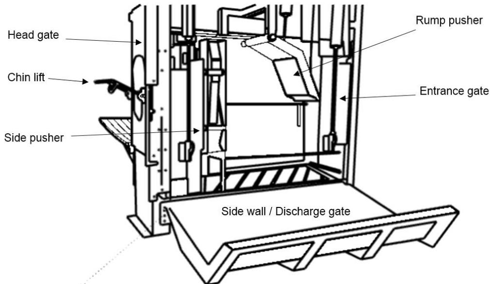
Figure 3 - Simple box with active restraint
