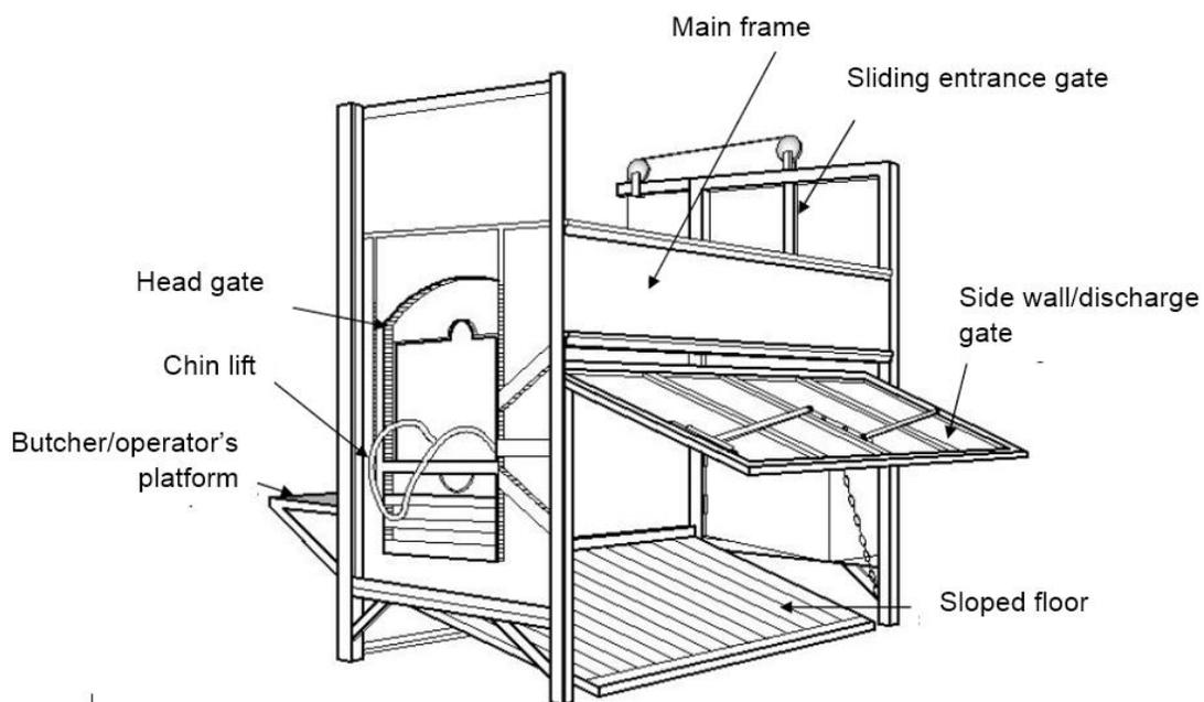
Figure 2 - Simple box with passive restraint
