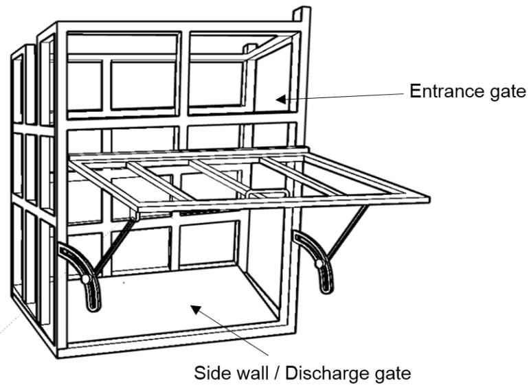
Figure 1 - Simple box large ruminant restrainer
